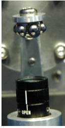
Figure 2: Omnidirectional camera with compound spherical mirrors
